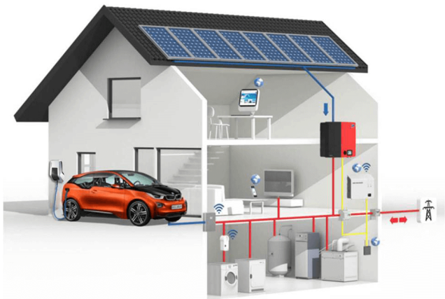
Smart controls and demand response measures in the home (Source: SMA Solar UK)
