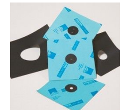
Airtightness grommets need to be used so that service penetrations do not increase air permeability (Source: Pro Clima)
