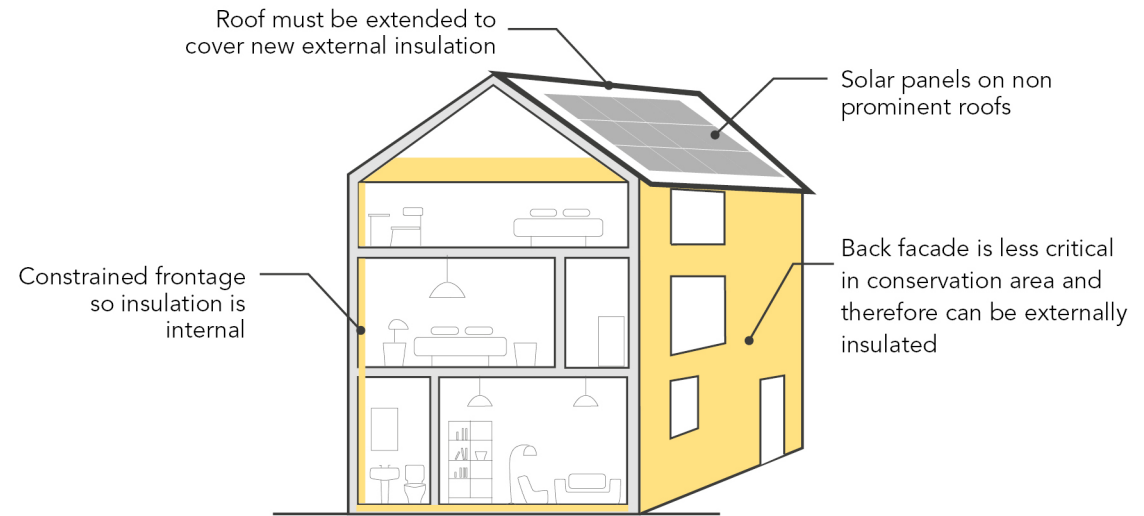
Diagram illustrating a hybrid retrofit approach with internal and external insulation.
